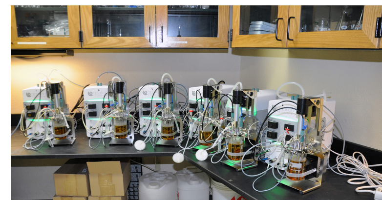
Six bench-top fermenters installed in a WIST lab at UW-Stevens Point allow simultaneous testing with multiple parameters.
