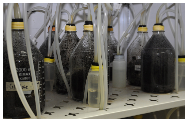
During the biodegradation trial for compostability testing, material is kept in closed vessels in a temperature-controlled environment.
