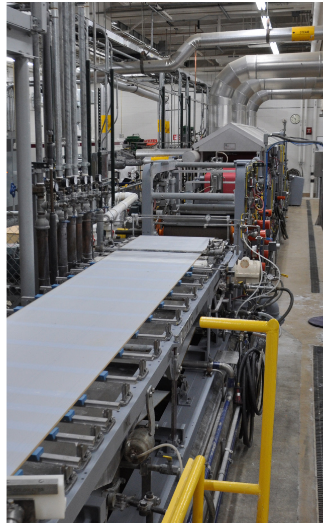
The pilot paper machine at UW-Stevens Point is used not only to train students in the paper science and chemical engineering program but for trial and small-scale production runs by WIST laboratory staff.
