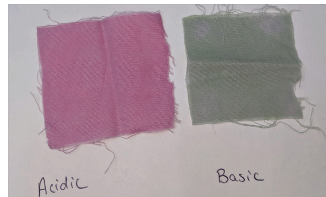
Fabric swatches colored with dyes made by WIST from cranberry processing residuals.
