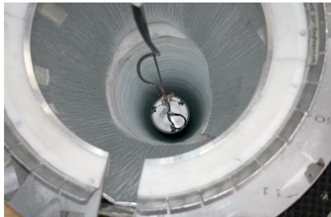
DM-Ice being lowered 2450m into the drilled ice
