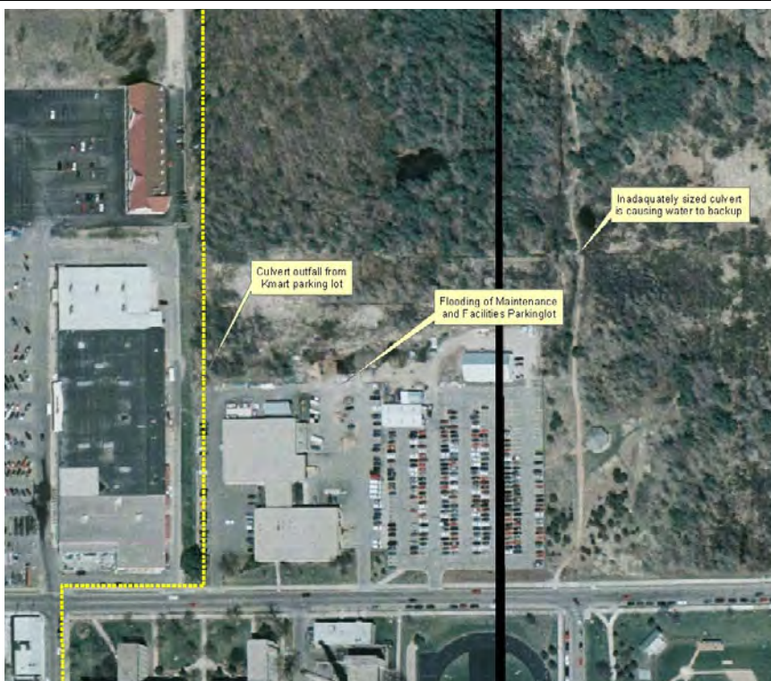
Figure 3-13 - Existing drainage problems
