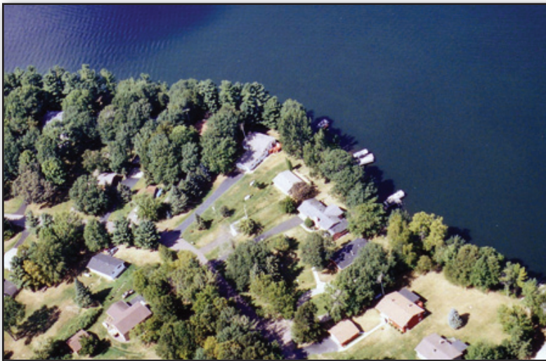
Dense, urban-scale development near lakes increases impervious surface, runoff, and nutrient delivery to lakes.
