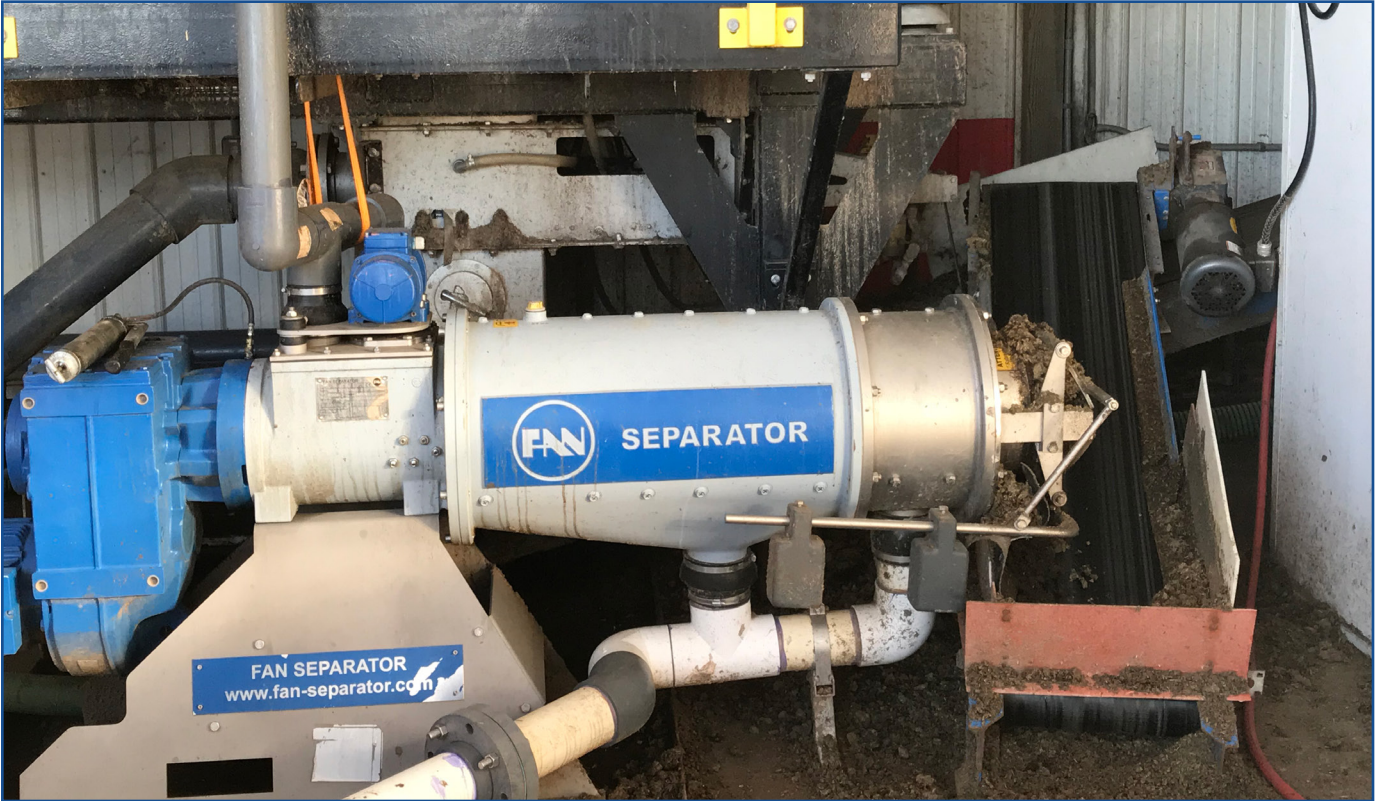
Photo 6: Feedstock separator at a dairy digester, Clean Fuel Partner, LLC
