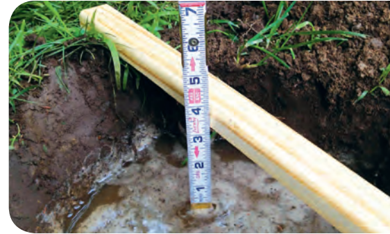
A simple perc test is performed to determine how well the soil will absorb and infiltrate runoff.
