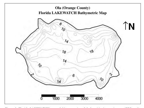
Figure 1. Florida LAKEWATCH created this map using global positioning equipment (GPS) and a depth sounder. Data were collected on October 10, 2006. Scale and map contours are in feet and were generated using Kriging technique in Surfer, a software package (Golden, CO). The center of the lake is located at Latitude 28°45'16" and Longitude 81°38'56". On this date, the lake surface area was calculated at 461 acres.
