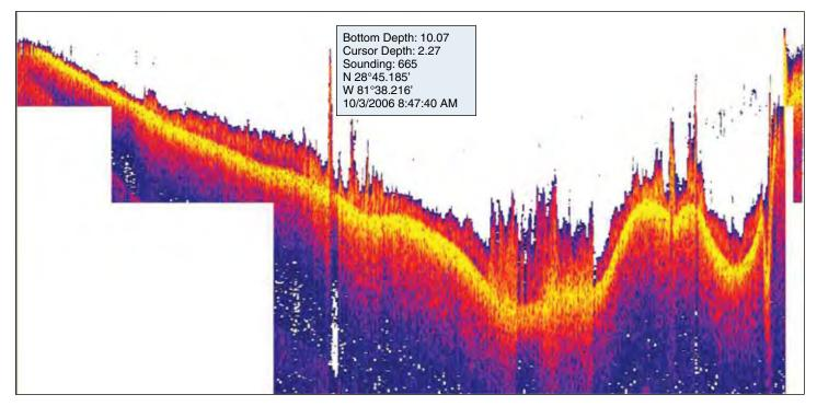
Figure 3. Depth sounding transect of Lake Ola taken October 10, 2006 using a Lowrance LCX-28CHD. The picture is captured from a computer as the transect is viewed with a program called Sonar Viewer. The hard bottom of the lake is shown in yellow while the submersed aquatic plants show in red above the yellow.
