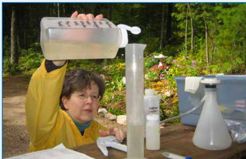
Pam McVety measures water she collected from Lake George to measure phosphorus levels and chlorophyll-A concentrations (a measure of algae growth in the water).
