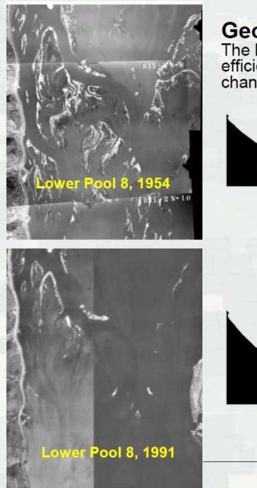
Geomorphic Response The backwaters became a very efficient flow path resulting in secondary channel erosion
