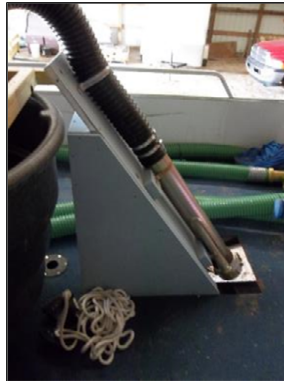
The water jet is mounted on a sliding board that can be raised for trailering
