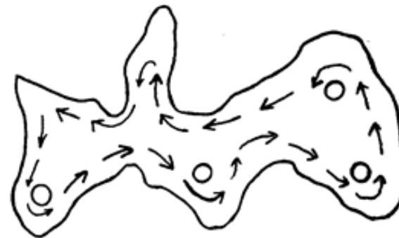
FIGURE 2. Example of boat route needed to survey an irregularly shaped lake.
