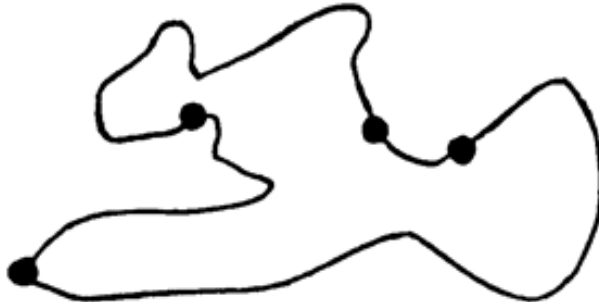
FIGURE 1. Example of vantage points needed to survey an irregularly shaped lake from land
