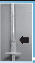
**STEP 6.** Insert the syringe into the hole in the cap of your glass vial containing your "fixed" sample. Very slowly, add the sodium thiosulfate solution drop by drop by pushing on the plunger of the syringe. Gently swirl your sample after each drop. It is possible to add as little as 0.1 units (half the distance between the lines on the syringe) with each addition.
