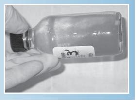
**STEP 12.** Once the precipitate has settled for a second time, add eight drops of sulfuric acid  $(H_2SO_4)$  from the squeeze bottle. Cap your sample bottle and invert to mix. Continue mixing the bottle for several minutes until all the precipitate has dissolved. The sample is now "fixed", meaning that the dissolved oxygen concentration cannot change.
