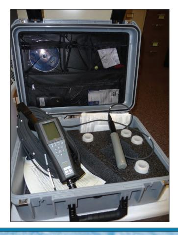
After sampling, it is very important to rinse and thoroughly air dry all of the equipment that you used. As always keep paperwork and envelopes separate from equipment. Be sure to turn off your meter and store out of direct sunlight.
