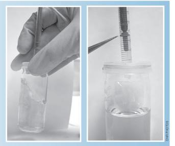
**STEP 14.** Rinse the syringe with distilled water and wipe it off before repeating steps 1 through 13 for your next sample. Remember, since this analysis only uses 20 ml of your "fixed" sample, if at any time you feel that you made a mistake, you should have enough "fixed" sample water remaining to repeat the analysis.
