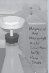
**STEP 6.** Carefully place the magnetic cup on top of the filter base. Be sure that the filter does not move! If the filter moves, wrinkles, or tears, remove the filter cup and discard the torn/wrinkled filter. Repeat steps 4 and 5 with a new filter.
