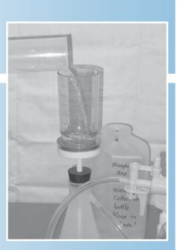
**STEP 10.** Squeeze the hand pump to move the water through the filter. Once all the water has been filtered, wash down the sides of the graduated cylinder and filter cup with distilled water to ensure that all of the algae are washed onto the filter paper.
