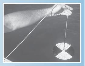
**STEP 5.** When the Secchi disk barely disappears from your view, mark the rope at the surface of the water with a clothespin.
