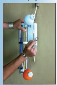
**STEP 4.** Release the arming pin to hook the loop (figure 4►).
