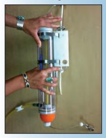
**STEP 2.** Start with the top seal (the rubber ball with the lanyard coming out of the top). Use your index finger to pull the arming rod of the release mechanism downward. Pull the top ball seal out of the sampler cylinder using the lanyard loop (figure 2▼).
