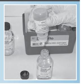
**STEP 9.** Then add eight drops of the alkaline potassium iodide azide solution. Once again, make sure to hold the squeeze bottle completely vertical (i.e. not at an angle) for consistent drop size and to avoid splattering.
