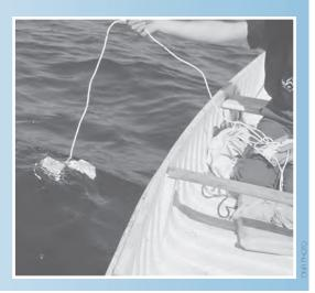
STEP 7. Bring the Secchi disk back into the boat.
