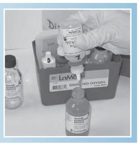
**STEP 10.** Cap your dissolved oxygen bottle and mix your sample by inverting the bottle 10 to 20 times. Put the bottle in the sample tray and allow the precipitate (e.g. the solid substance that is forming in your bottle due to a chemical reaction) to settle. This process may take a few minutes.
