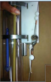
**STEP 5.** Arm the bottom seal (the rubber ball) using the same procedure as above and clip the stainless steel clip around both strands of the loop lanyard (figure 5►).
