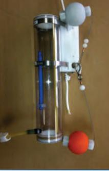
**STEP 8.** After sampling, thoroughly rinse your sampler with distilled water. Place pencils in either end so the sampler will dry out. Open up or remove the hose clamp so the hose will air dry as well. When the sampler is dry, remove pencils so the rubber tubing does not stretch and wear out.
