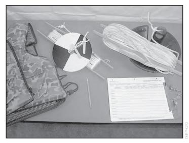
After sampling, it is very important to rinse and air dry thoroughly all of the equipment that you used. Keep paperwork separate from equipment.
