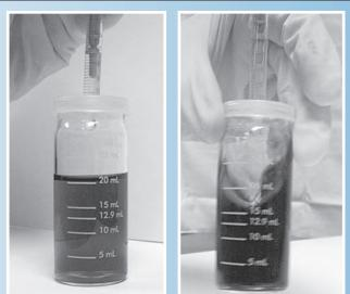
**STEP 13.** When your sample has turned clear, remove the syringe. Before expelling the remainder of the sodium thiosulfate solution in the syringe, read and record the volume of solution that you used (see "Reading the Syringe" on the next page).
