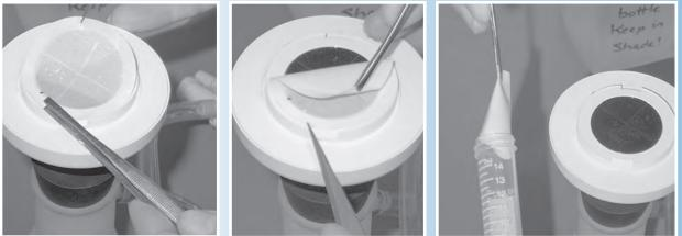
**STEP 13.** Fill out the chlorophyll label and place it on the tube containing your chlorophyll sample. Be sure to include the volume filtered (mls) on the label. Your station id number should be written on the label.
