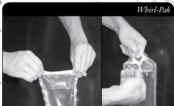
Step 1: Fold the top of the Whirl-Pak 4-5 times.
