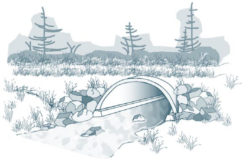
Figure 5. An open-bottom culvert
