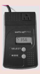
A watt meter is an electronic instrument that measures the power (watts) used by an appliance. When you plug the appliances into your meter, you can measure how much electricity your appliances are using and what they are costing you. The meter will display wattage, cumulative kilowatt hours and cumulative cost. There should be an instruction guide that accompanies the meter for details in using the various functions.
