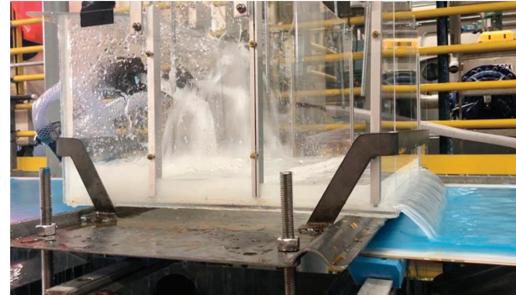
A secondary headbox built by a paper science and engineering senior design team (see story page 12) adds new laboratory services and research capability. Paper pulp is shown exiting the headbox on the right side.
