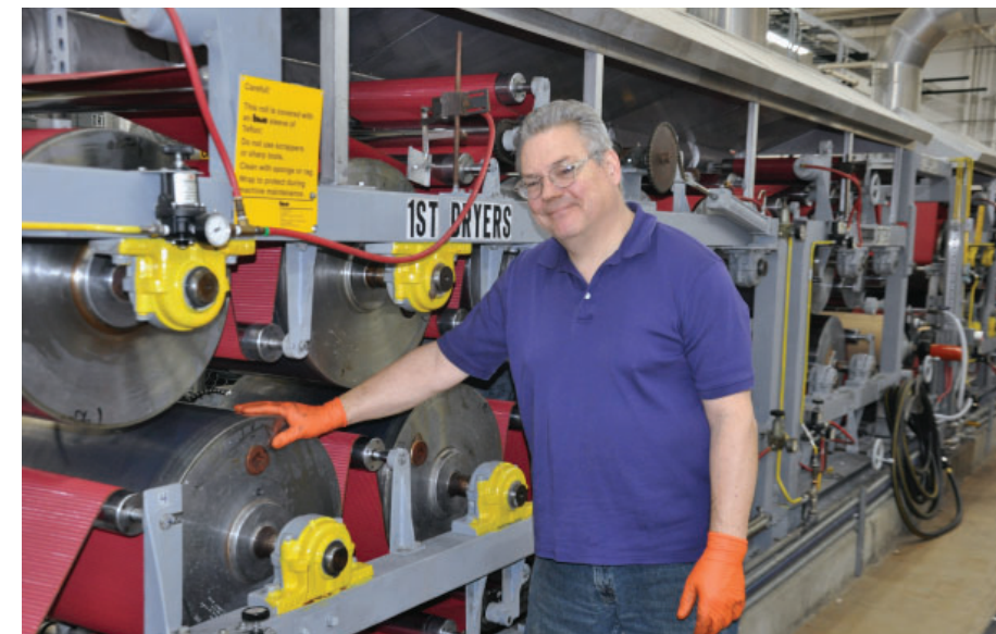
Brian Bandow, WIST paper machine and laboratory specialist, indicates the new Teflon sleeves installed on dryer cans on the university’s pilot paper machine.
