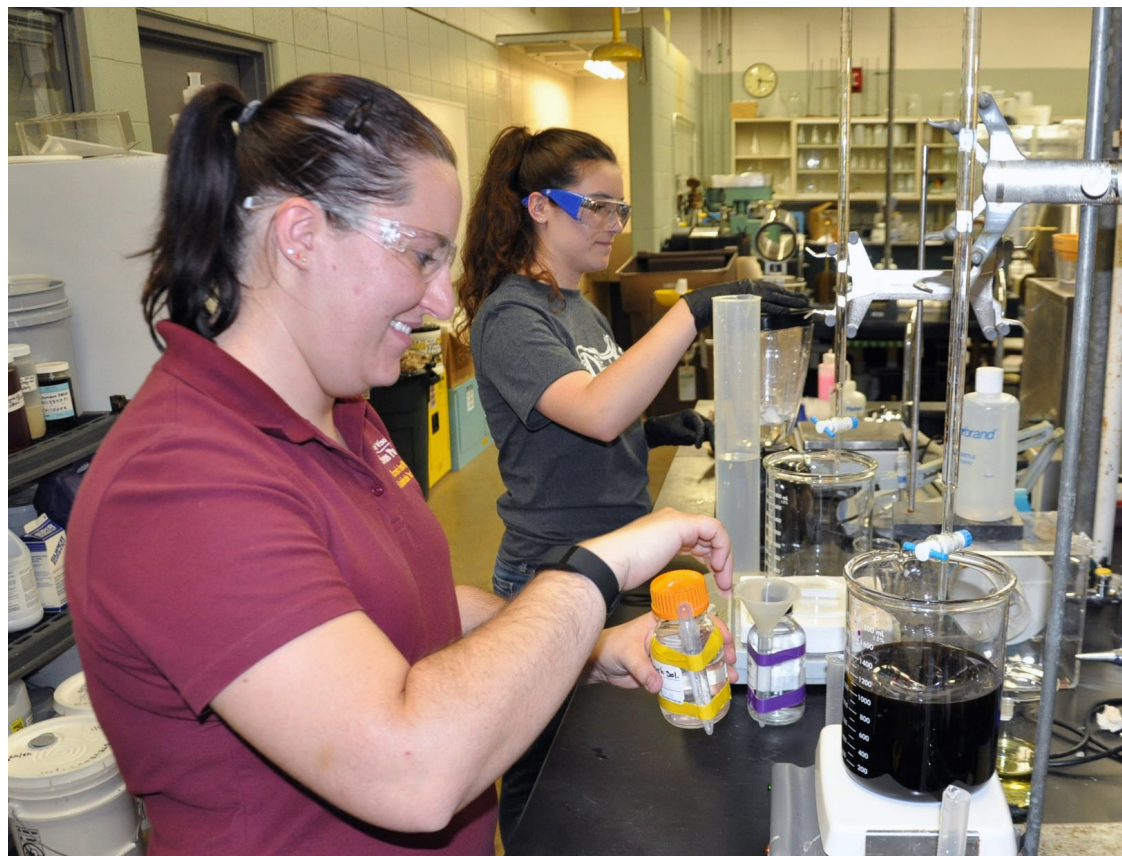
Lindsey Hoffman, WIST papermaking and laboratory projects specialist, performs a lab test to determine the lignin content of paper sent to WIST for analysis. Katie Ebelt, in background, a Paper Science and Engineering student employed by WIST, pulps another sample of the paper for an additional trial.
