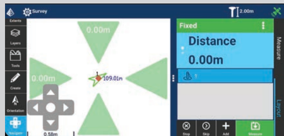
Sub-meter guides provide fast, precise staking
