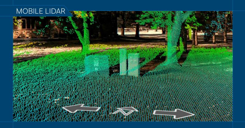
obile lidar is revolutionizing how departments of transportation survey transportation corridors, as well as supporting a wide range of other engineering applications. It achieves survey-grade accuracies for design and as-built surface modeling, it performs systematic inventory of transportation assets, and it facilitates clash detection and clearance measurements for bridges and overhead obstructions.
