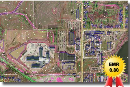
Topographic mapping is required by a wide variety of clients and is needed to show all manmade, non-terrain and terrain features into a printed or CAD mapping format. Our staff compiles these features from aerial photographs under the direction of ASPRS-certified photogrammetrists. Map scale and contour intervals are determined prior to the aerial photographic mission and are then compiled to meet the required mapping accuracy.
