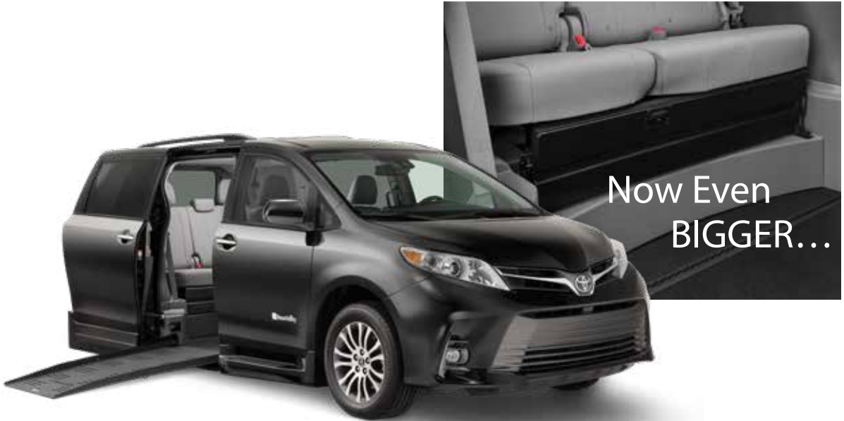
Side-Entry Conversion with power fold-out ramp
