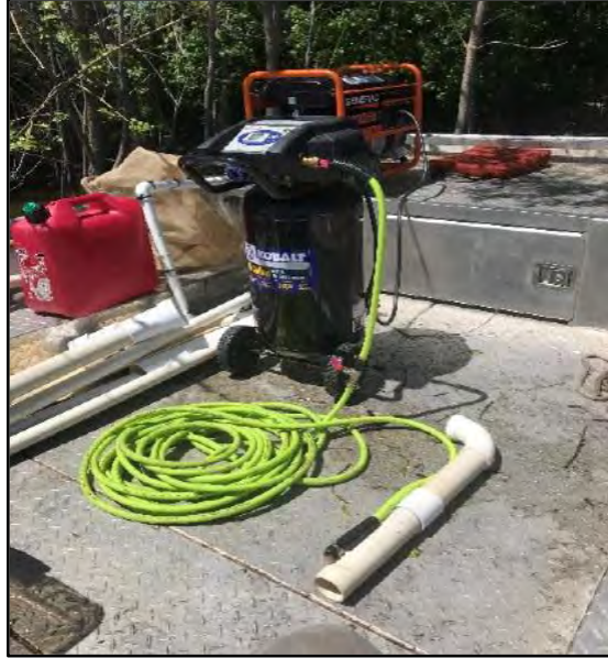
Figure 11: Our airlift pump, which consisted of a generator, air compressor, air hose, and PVC pipe.
