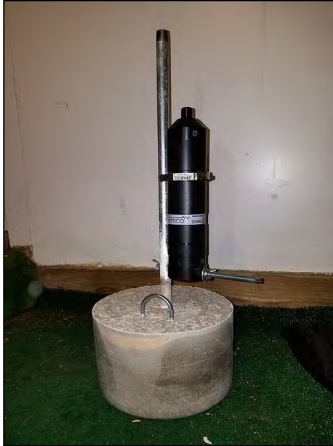
Figure 8: In tributaries, each VR2W acoustic receiver was attached to a steel pipe encased in a concrete block, submerged 20 m offshore, and secured to onshore trees with a chain.
