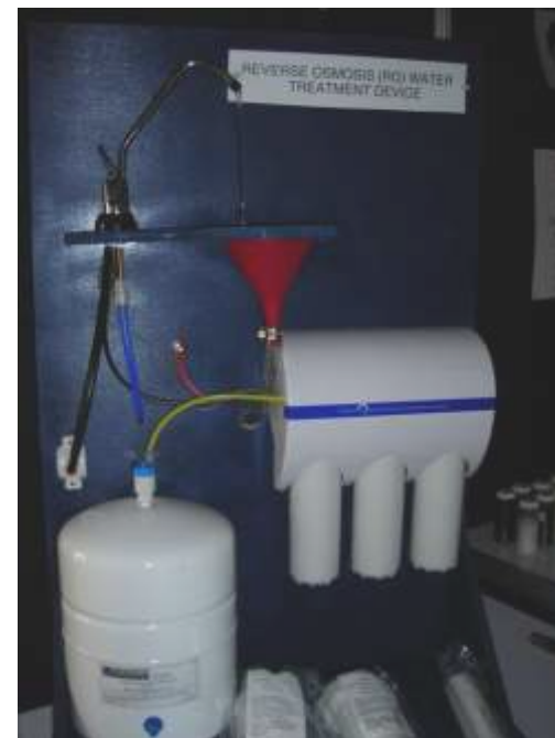
Example of a reverse osmosis (RO) water treatment technology. It is a point of use method commonly used to treat water for drinking and cooking.
