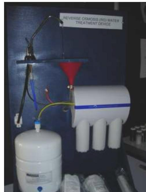
Example of a reverse osmosis (RO) water treatment technology. It is a point of use method commonly used to treat water for drinking and cooking.
