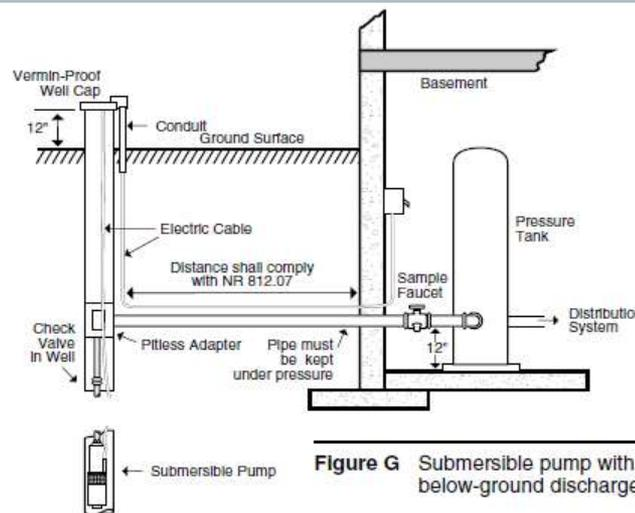
Figure G Submersible pump with below-ground discharge
