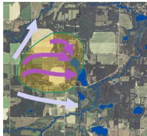
Figure 2. Groundwater contribution area to Stratton Lake. (courtesy of P. McGinley)
