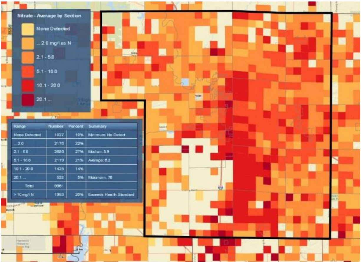
Figure 12. Nitrate-nitrogen concentrations by section for historical well water sampling data in Portage County. Samples represent data from the WI Well Water Quality Viewer (CWSE, 2018). Spatial patterns of nitrate concentrations are similar to those observed in the current study of nitrate (Figure D). Blank cells represent areas with insufficient data.
