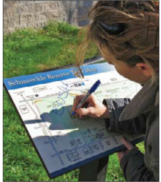
High-pressure laminate panels are resistant to most forms of graffiti, including permanent markers (above), spray paint, lipstick, and crayons. Marks can be removed with organic solvents or mineral spirits.
