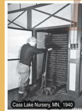
Cones on screen trays were heated in a *forced-air kiln* for 8 to 16 hours to open their scales.
