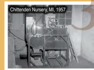
The seeds were placed into a *dewinger* machine that rubbed off the seed wings and scales.
