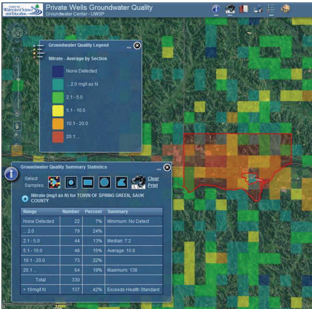
Figure 2: The interactive well water quality viewer generates color-coded maps for common water quality descriptors. Data can be accessed at the county, town, section, watershed or other user-defined scale.
