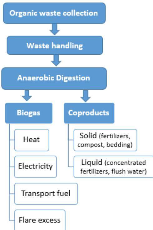
Figure 2: Biogas production steps, process and uses (Adapted from EPA AgStar)<sup>1</sup>
