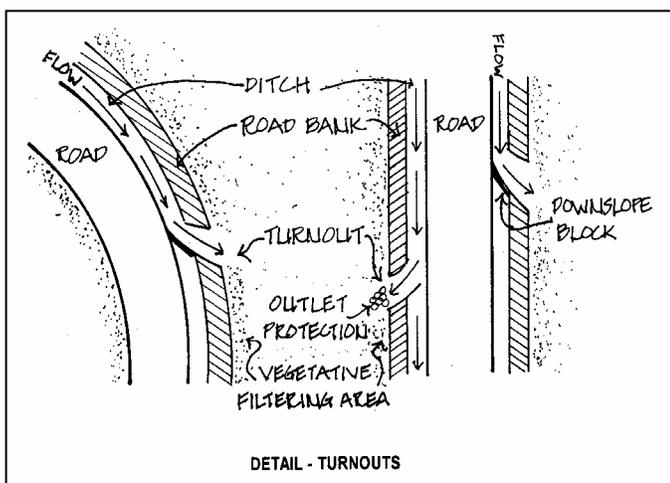
Turnouts should be stabilized so as not to create additional soil erosion. The turnout can be seeded and stabilized with hay mulch or erosion control blankets. Alternately, on steeper slopes or areas receiving greater flow, 3"-6" angular stone rip-rap placed over non-woven geotextile fabric can be used to line the structure.
