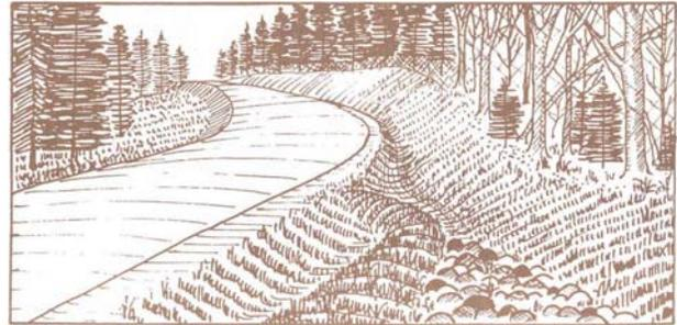
Turnouts return stormwater runoff as sheet flow to natural drainage areas. Often turnouts are simply extensions of ditches that redirect water into the woods and disperse runoff before it can cause erosion. Turnouts reduce the speed of runoff, allowing soil particles to settle out instead of being transported to a stream, river, or lake. Water and nutrients can then be filtered and absorbed by the surrounding vegetation.
