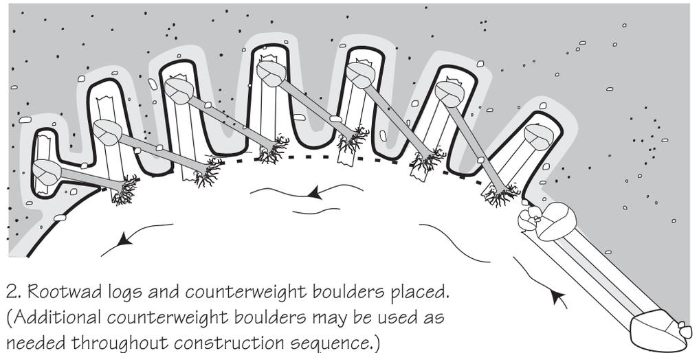
2. Rootwad logs and counterweight boulders placed. (Additional counterweight boulders may be used as needed throughout construction sequence.)
