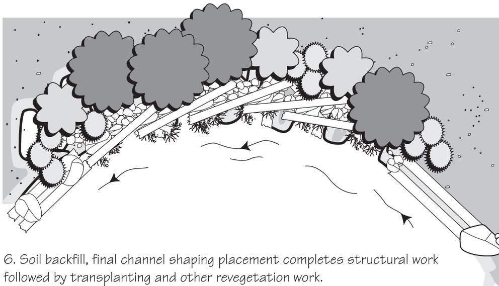
6. Soil backfill, final channel shaping placement completes structural work followed by transplanting and other revegetation work.
