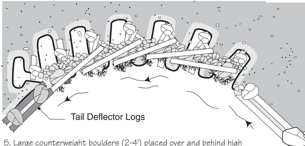
5. Large counterweight boulders (2-4') placed over and behind high stage deflector logs, followed by placement of smaller, cut-off rock (4"-12"). Tail deflector logs placed.
