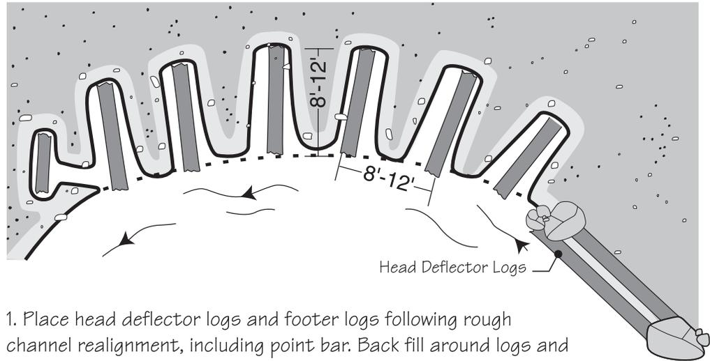
1. Place head deflector logs and footer logs following rough channel realignment, including point bar. Back fill around logs and or rock after each sequence.
