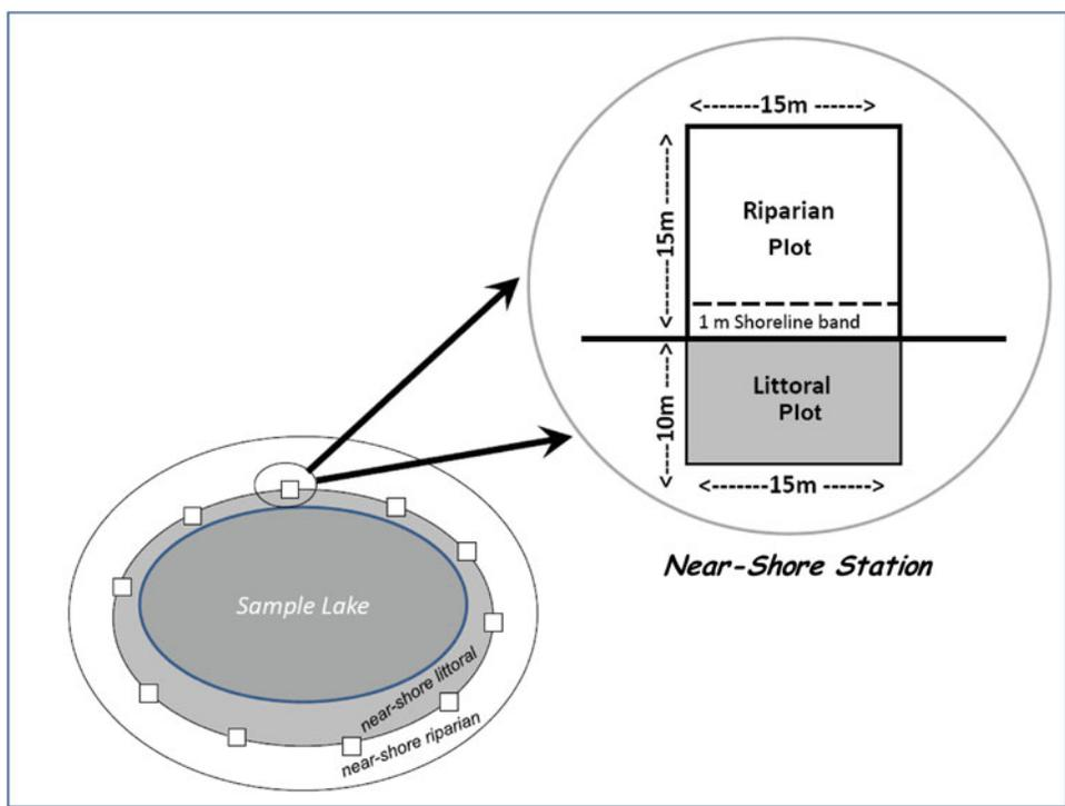
**Figure 2.** Field sampling design with 10 near-shore stations at which data were collected to characterize near shore lake riparian and littoral physical habitat in the EMAP-Northeastern Lake Survey. The 10 stations were systematically spaced around the shore of the lake from a random starting point. Insert shows riparian plot, shoreline band, and littoral plot located at each station.
