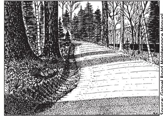
Crowned driveway with a rock-lined drainage ditch.
