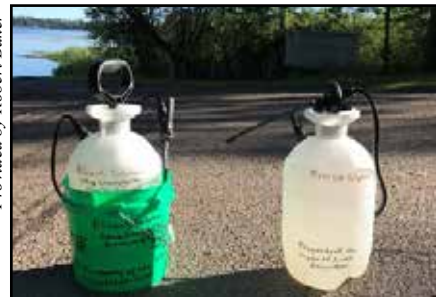
Pump Sprayer Shielded in Two-gallon Plastic Bucket
