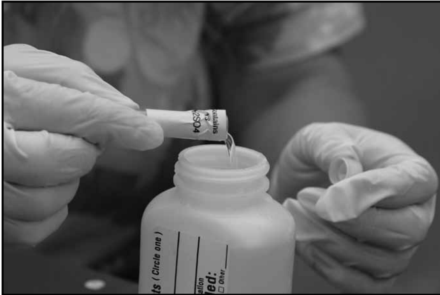
Testing a blank phosphorus sample to assure no residual phosphorus is in the equipment.
