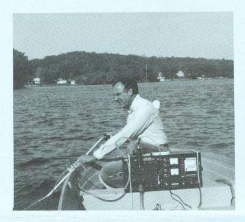
The photograph shows the Lauderdale septic leachate detector system in action. Groundwater entering the lake near the shoreline is continuously drawn to test conductivity and fluorescence. Simultaneous high conductivity and fluorescence readings are an indication of local septic failure. Correlation has subsequently been obtained with fecal bacterial sampling.
