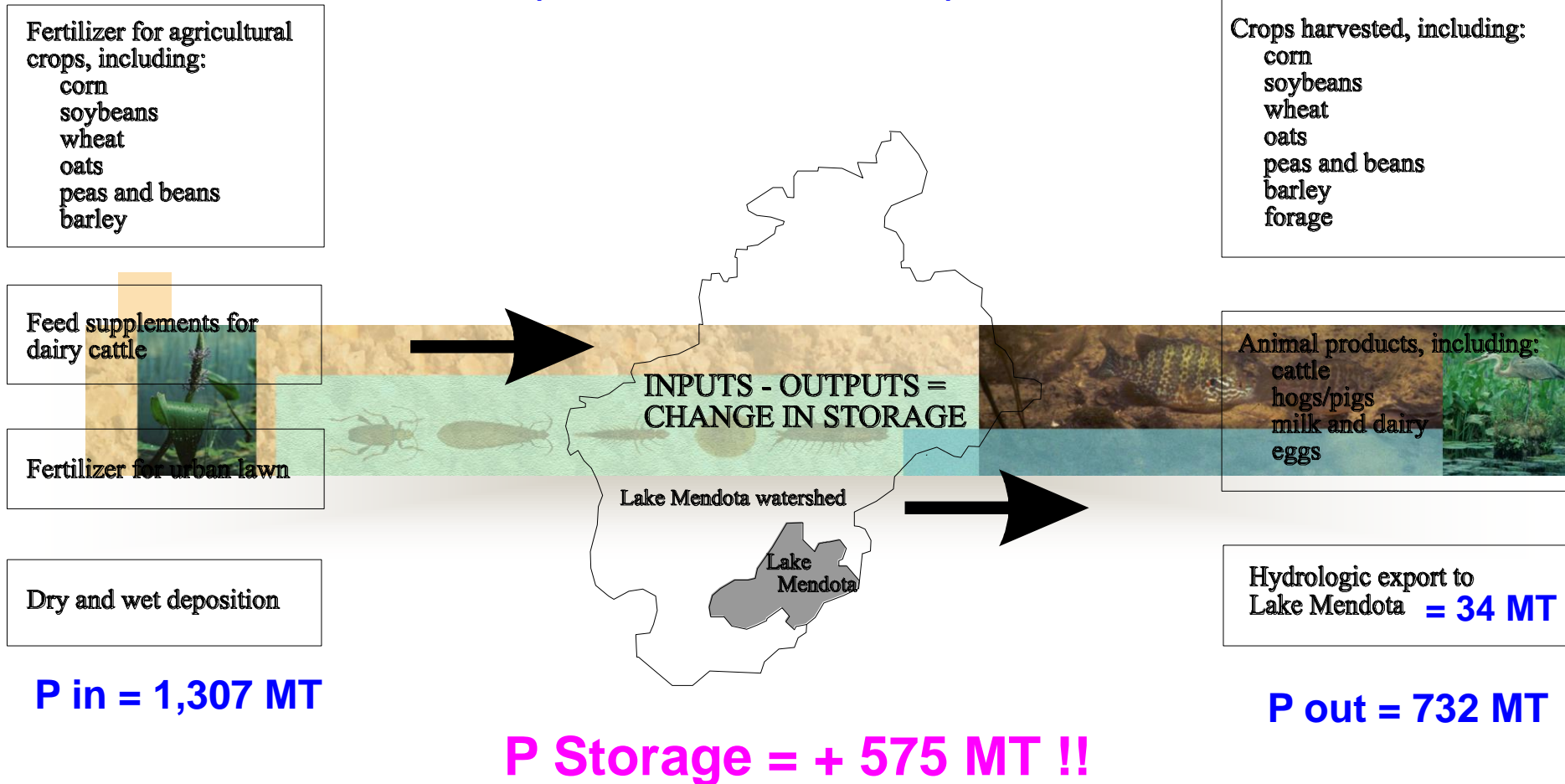
Figure 1. Schematic diagram of inputs and outputs used to calculate a P budget for the Lake Mendota watershed for 1995.
