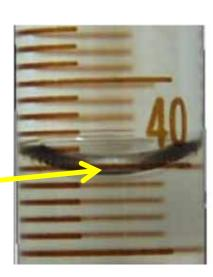
As water fills up the measuring tube, a curved surface is formed called a meniscus. It is formed by the surface tension of a liquid in contact with the sides of the tube.
