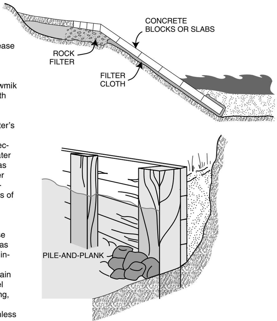
**Figure 2.** Solid retaining walls (seawalls) built of concrete (top) or wood (bottom). Adapted from Rogers, Golden and Halpern, Inc., U. S. Army Corps of Engineers (1981).
