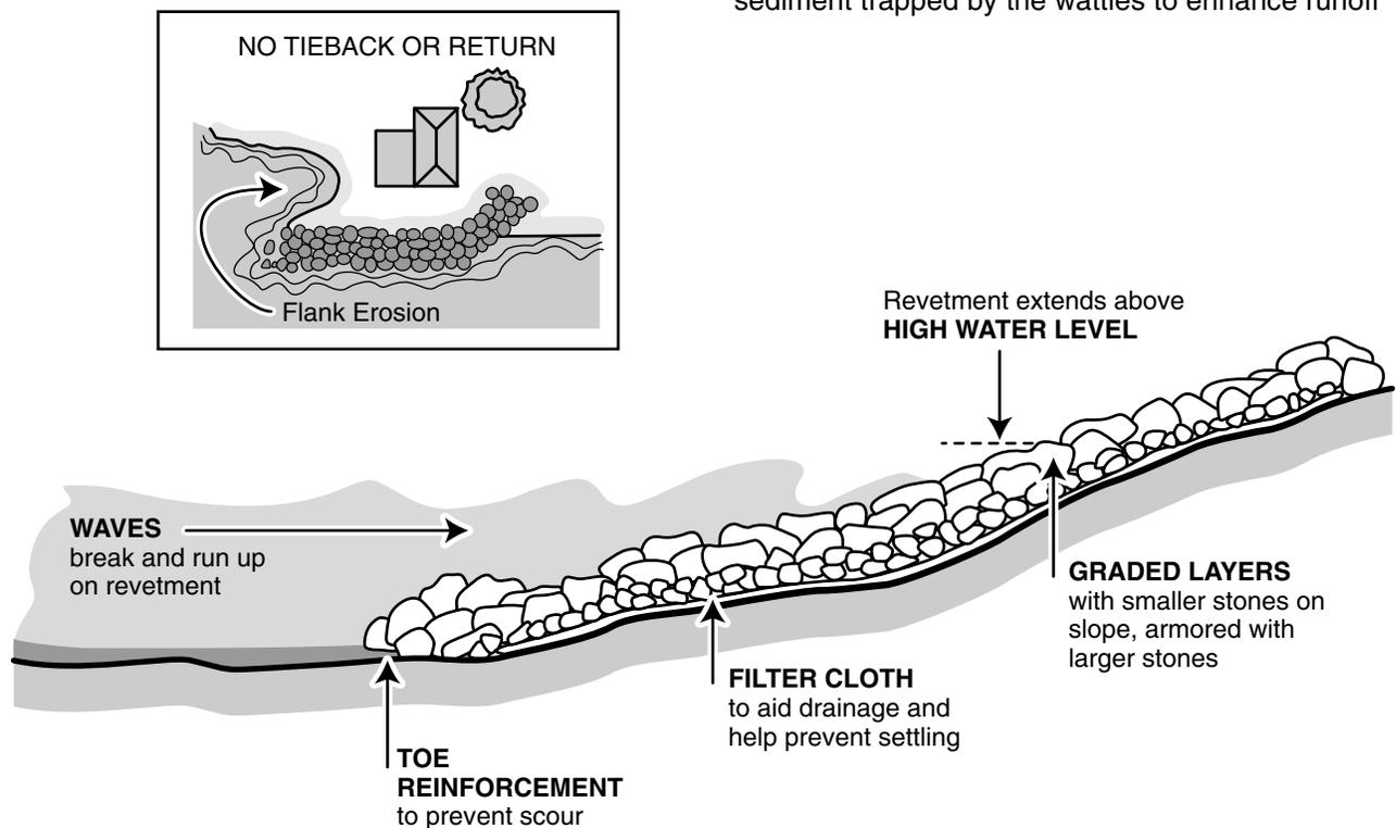
**Figure 1.** Bouldery riprap diagramed to show wave action in relation to flank erosion (top) and construction layers (bottom). Adapted from Rogers, Golden and Halpern, Inc., U. S. Army Corps of Engineers (1981).
