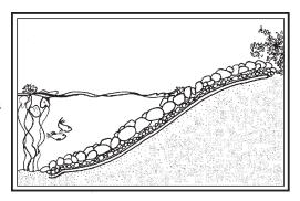
shoreline, use of pea gravel (small rounded stones about 1/4 inch diameter) is the only allowable material because it will provide more stability than sand in eroding or unstable areas.
