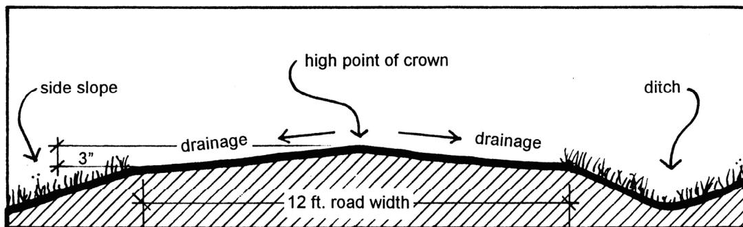
A properly crowned road or driveway allows water to flow immediately off the road into surrounding vegetation or a stabilized ditch. Water running lengthwise down the road is likely to cause erosion of the road surface.
