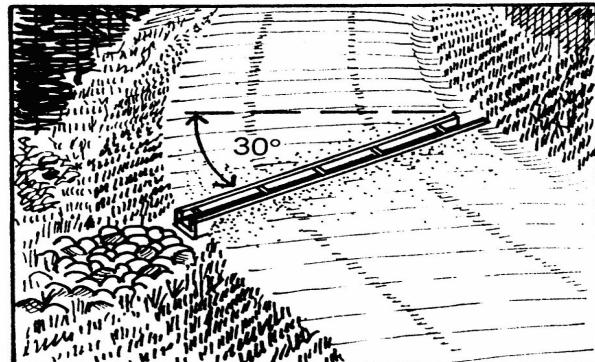
An open-top box culvert is an alternative to a waterbar that will hold its shape better. Be sure to make it wide enough to allow periodic cleaning out with a tool you have such as a mattock. Install both waterbars and open-top culverts at a 30° angle to the road width. Note the rock apron at the culvert outlet above to prevent erosion at this location.
