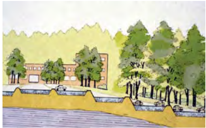
Figure 7.37 Slope stepping with berms
