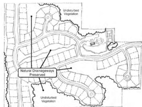
Schematic of a site design protecting natural drainage features Source: Georgia Stormwater Management Manual, Volume 2: Technical Handbook, First Edition. August, 2001
