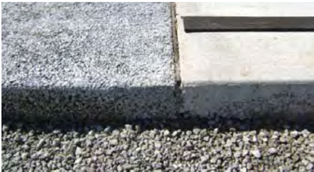
Pervious and impervious concrete
