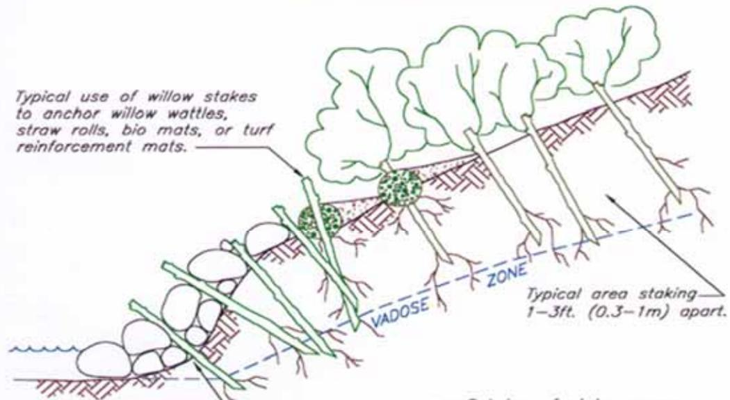
Typical — drive or plant willow stakes through openings in riprap or gabions.
