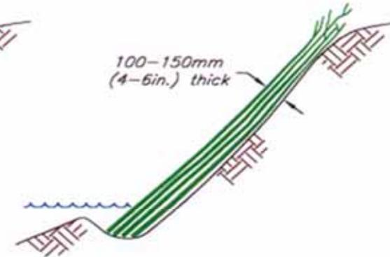
Step 2: Place willow branches making sure that the butt ends reach the bottom.
