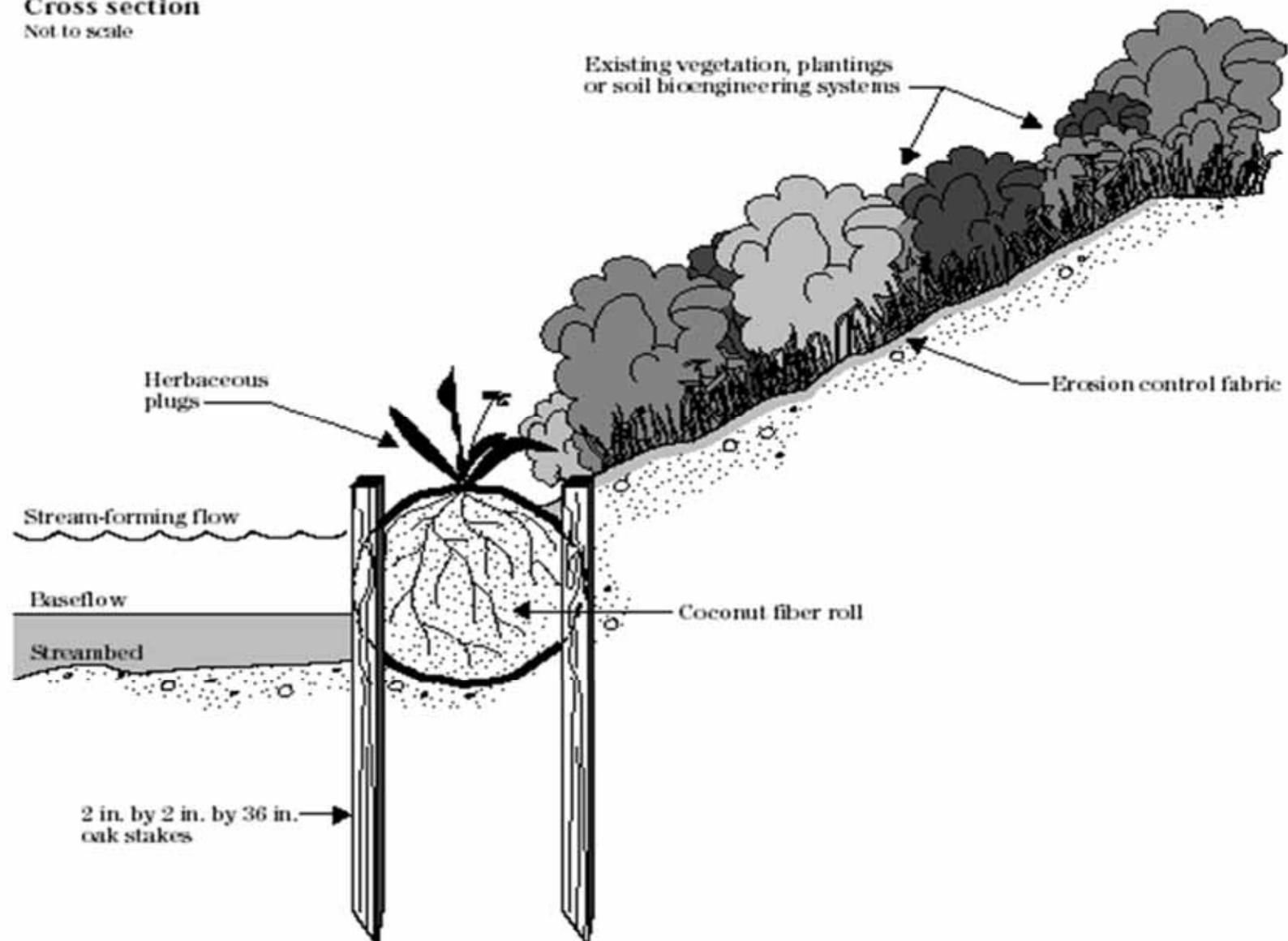
**Figure 16-56** Coconut fiber roll details
