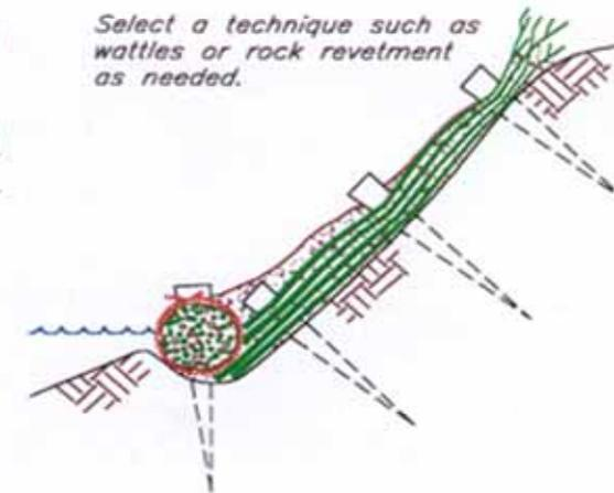
Step 4: Drive the stakes deeply into the bank to tightly compress the branches against the soil. Cover and partially bury the mattress to encourage rooting.
