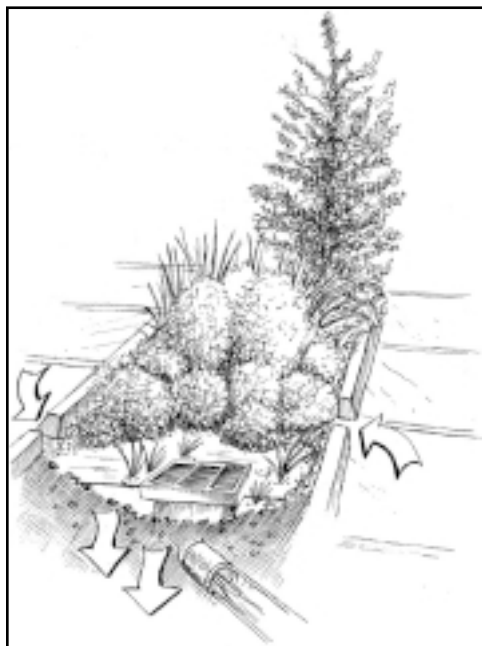
INFILTRATION SWALE (ADAPTED FROM CITY OF PORTLAND)
