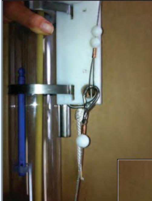
**STEP 5.** Arm the bottom seal (the rubber ball) using the same procedure as above and clip the stainless steel clip around both strands of the loop lanyard (figure 5▶).
