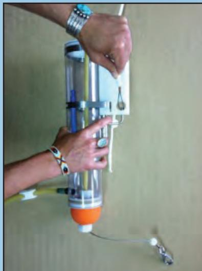
**STEP 3.** Insert the lanyard “loop” inside the hole in the closing mechanism. Release the arming pin to hook the loop (figures 3 ▼).
