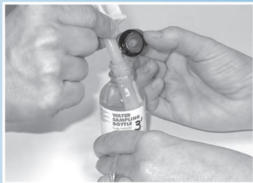
**STEP 5.** While the water is still flowing, slowly remove the tube allowing your sample bottle to overfill. Water will actually appear above the top of the bottle.
