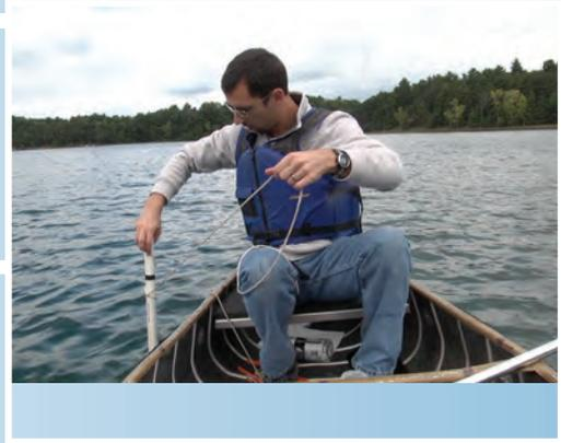
**STEP 4.** Drain the integrated water sampler by touching the collection end of the sampler to the rod in the neck of the water collection bottle. Water will drain from the integrated water
