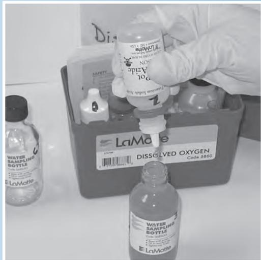
**STEP 10.** Cap your dissolved oxygen bottle and mix your sample by inverting the bottle 10 to 20 times. Put the bottle in the sample tray and allow the precipitate (e.g. the solid substance that is forming in your bottle due to a chemical reaction) to settle. This process may take a few minutes.
