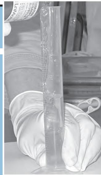
**STEP 3.** Pour the 20 ml sample that you just measured from the graduated cylinder into the small glass vial. Cap the glass vial with the center-hole plastic lid. Please note that even though the glass vial may have volume measurement markings on it, the graduated cylinder is a more accurate measure of volume than pouring your “fixed” sample directly into the small glass vial.
