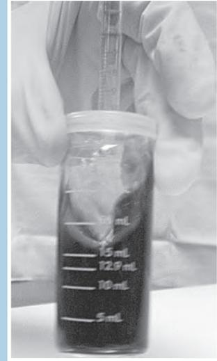
**STEP 13.** When your sample has turned clear, remove the syringe. Before expelling the remainder of the sodium thiosulfate solution in the syringe, read and record the volume of solution that you used (see “Reading the Syringe” on the next page).
