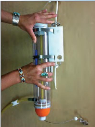
**STEP 2.** Start with the top seal (the rubber ball with the lanyard coming out of the top). Use your index finger to pull the arming rod of the release mechanism downward. Pull the top ball seal out of the sampler cylinder using the lanyard loop (figure 2 ▼).
