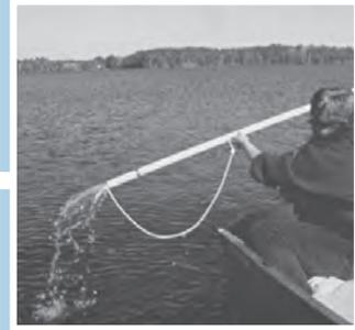
**STEP 2.** Rinse the water collection bottle and cap with lake water three times. Always place the cap top side down to prevent contamination of the inside of the cap.
