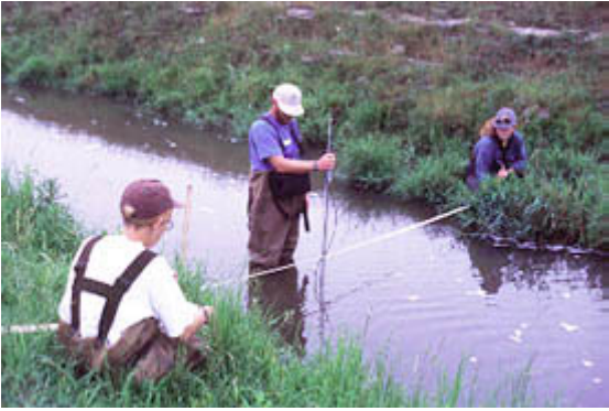
Measuring a stream's width, depth, flow rate, temperature, pH, dissolved oxygen and nutrient levels. © Mike Miller
