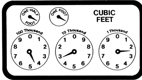
Somewhere on the meter are two dials by themselves. They are marked “one-half cubic foot” and “one cubic foot.” The gas company uses these to check the meters to be sure they are accurate. They are not used when reading the meter.
