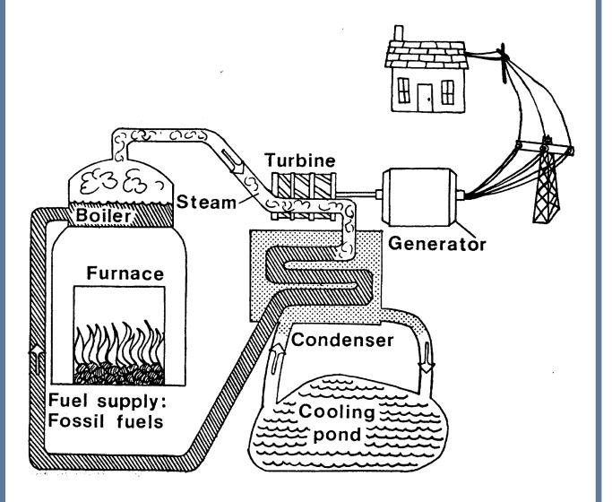
Fossil fuels (oil, gas, coal) produce electrical power when they are burned in a furnace to heat boilers that make steam. The steam turns a turbine, drives a generator that makes electricity.
